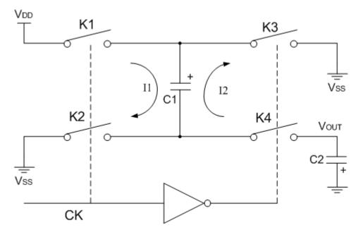
SMP7660 together with two external capacitors C1、C2 complement a voltage Inverter. Capacitor C1 is charged to a voltage  $V_{DD}$ , for the first half cycle when switches K1 and K2 are closed ( while switches K3 and K4 are open during this half cycle); During the second half cycle of operation, switches K3 and K4 are closed, with K1 and K2 open, thereby shifting capacitor C2 negatively to  $-V_{DD}$ .
